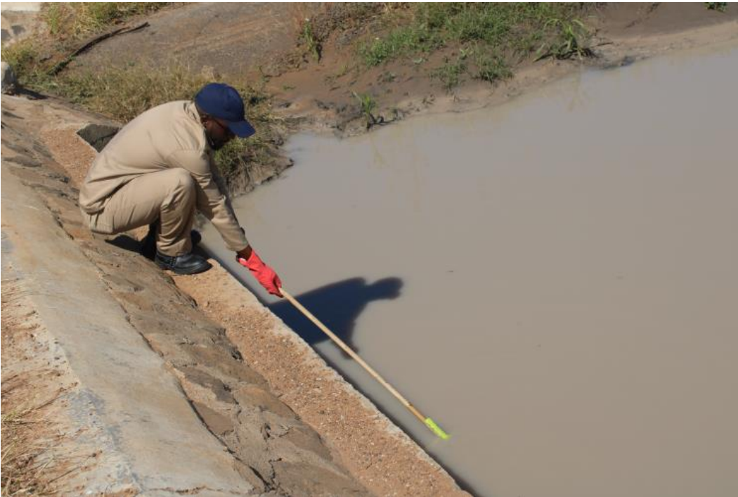
Plate 4: Collecting water samples from the sub-drainage channel during the first site visit
