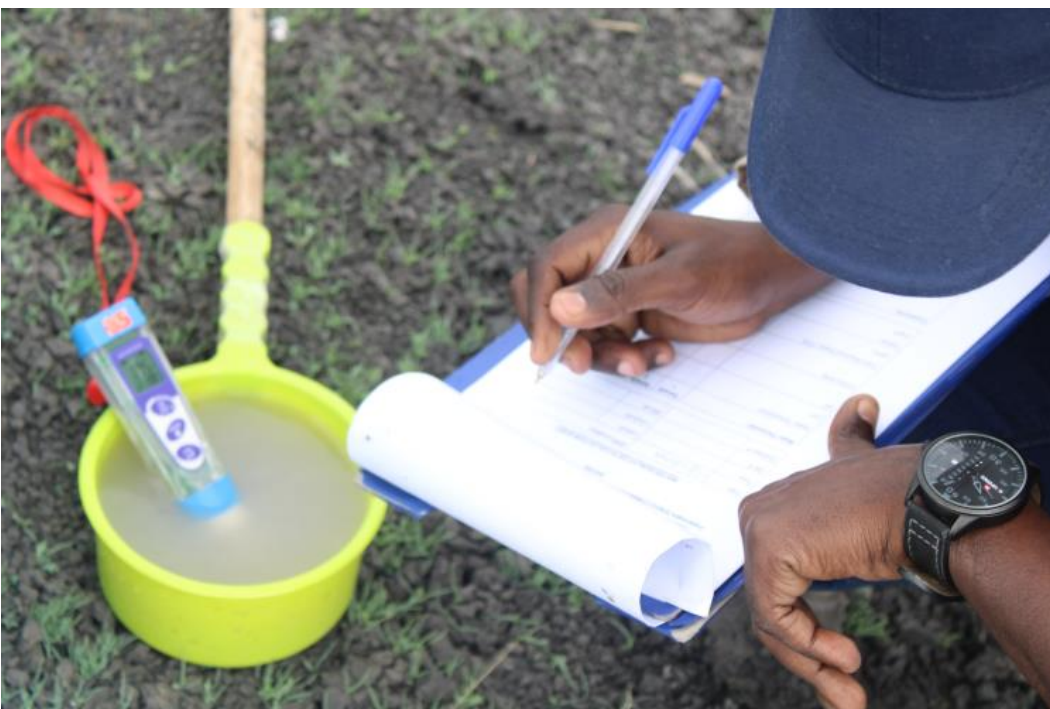
Plate 5: Taking onsite readings of the physical parameters using an XS PC-5 Multimeter Tester kit
